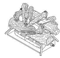
Figure 20 - Placement of Top Logs (Kingston Split Oak Logs Shown)
